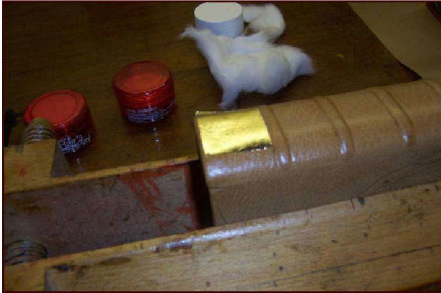
All things being equal, the leaf should adhere to the book as the book has more grease on it than the pad had, remove the pad and the leaf should be stuck in place, as shown above.
