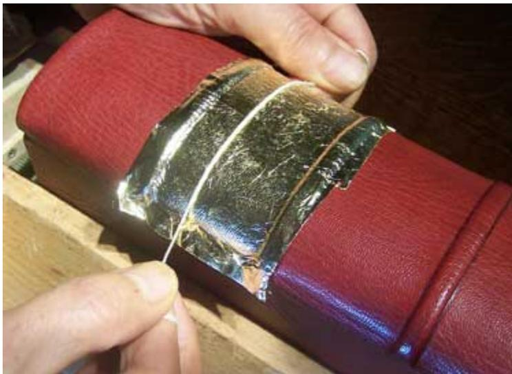
Sight the thread so that it is where you would like the top of your letters to be and then pull the thread down onto the leaf, give a slight sideways pull and you will find that the thread cuts through the leaf leaving a nice clean line which you can use as a guide when it comes to tooling in your lettering.
