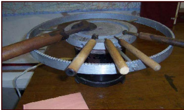
Now we come to another very important area of gilding...the temperature of the tools. To be precise a temperature of between 250 and 260 degrees Fahrenheit will do the job, to put it another way, using a Cockerel finishing stove like this one, the simmer setting is just right, bring the tools up to the simmer temperature and they are ready to use.
