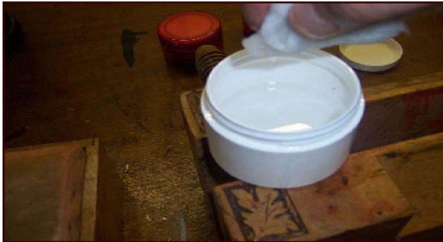
Having tooled all the areas of the book that were required, get a small pot of white spirit and dip a pad of cotton wool into the spirit, squeeze out most but not all of the spirit and wipe off the surplus leaf with the pad, do not rub the pad over the leaf, rather wipe over an area, remove the leaf, and then using a fresh part of the pad, wipe another area and so on, as shown below.
