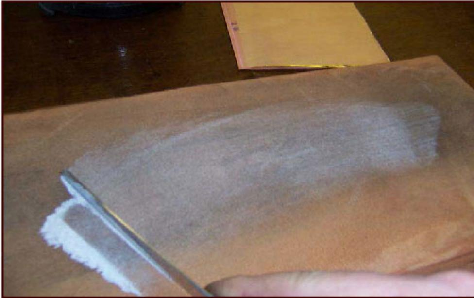
Next, spread the pumice over the face of the cushion, and wiping the knife back and forth distribute the pumice over the cushion, making sure that the knife gets wiped several times to remove any traces of grease from it; then with the knife, brush off all the surplus pumice.
