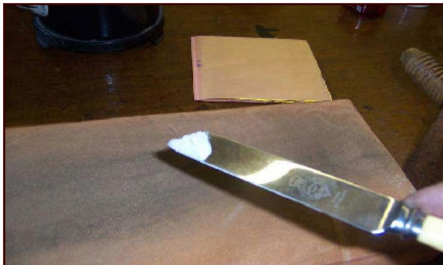
Using the gilders knife, scoop out a little of the pumice powder and deposit it on the cushion. Binders used to use a type of brick which they scraped powder from to degrease the cushion, but this type of brick is now either impossible to find or very expensive indeed, thus I have used fine grade pumice powder for many years as an inexpensive substitute.
